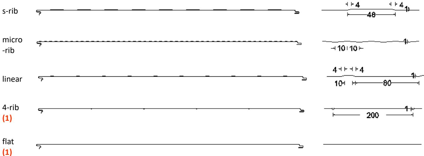
(1) The minimum allowed steel thickness for Flat & 4-Rib modulations is 0.6mm.
